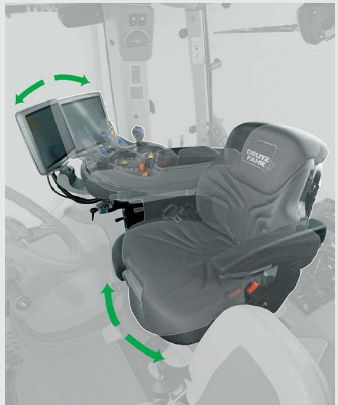
↑ Now available for all TTV models: Seat with up to 20° rotation for added comfort and ease of operation.
