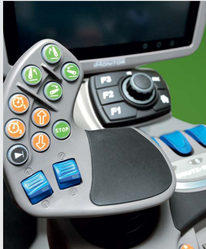
↑ With two buttons on the MaxCom multi-function joystick, the driver can use four different speed settings for field work or on the road and maintain a constant speed for optimum results.
