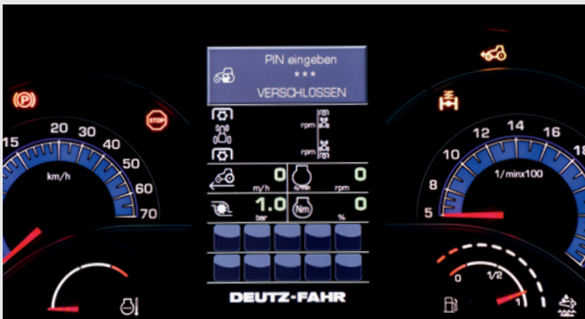
↑ State of the art dashboard with InfoCentrePro: 5" high-resolution colour display for customisable information concept at top level. The code lock in the tractor ensures security – lock and unlock with a PIN.
