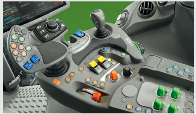
RCshift: Available as a variant with mechanical control devices as a variant with multifunction armrest, electro-hydraulic control valves and iMonitor.
