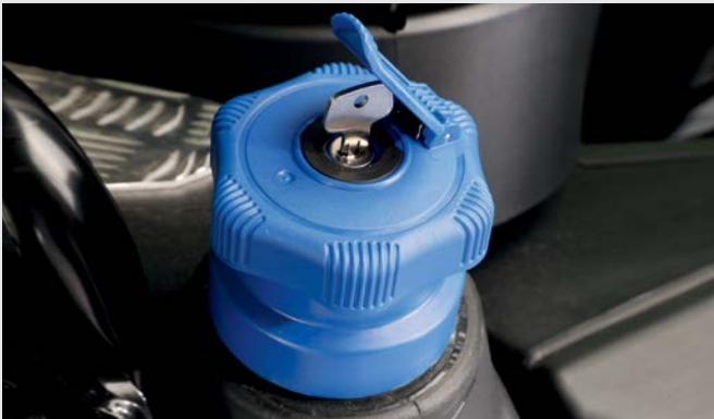
↑ Lockable tank covers for fuel and AdBlue tanks.
