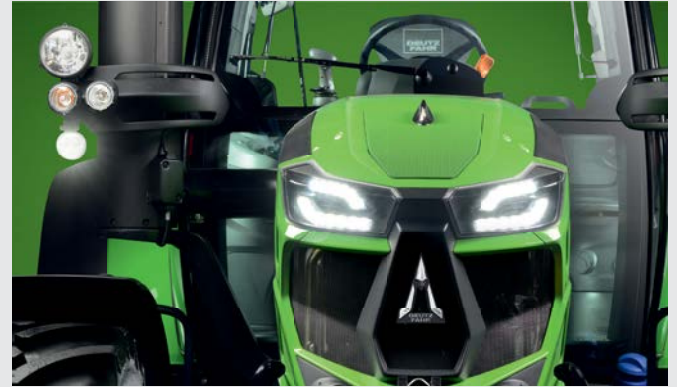
↑ LED package with up to 2,500 lm per work light (depending on the model).
