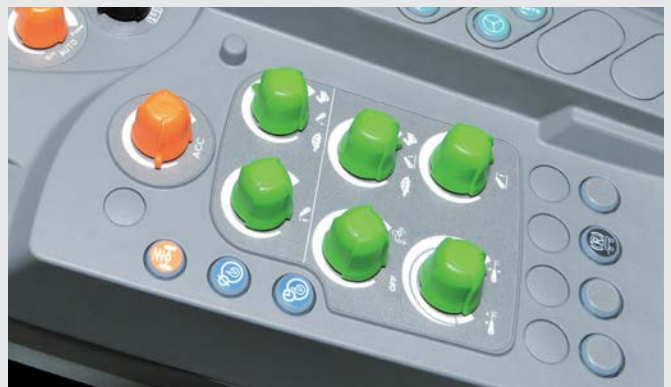
↑ The front linkage (TTV only) and rear linkage control can be fine adjusted with the potentiometer in the armrest.
