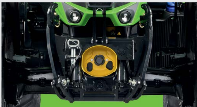
↑ Position controlled front linkage with up to 5,480 kg lifting power (TTV models).
