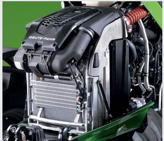
↑ PowerCore technology for the air filter: 20 % higher air flow capacity compared to standard filters.
