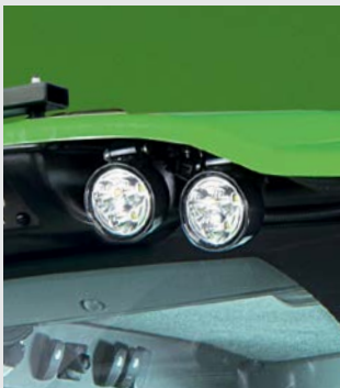
↑ Up to 16 LED work lights (generation IV, 2,500 lm per light).
