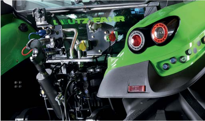
↑ The compressed air brake system decelerates trailers in all weight categories reliable and safely.
