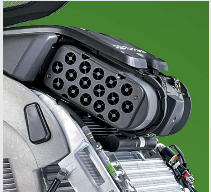
↑ Pre-cleaning system in the engine air filter: Spiral cyclone tubes and aspirator hoses remove 95 % of the dust before these can enter the primary filter.
