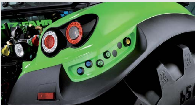
↑ Easy operation of the hydraulic system, rear linkage and PTO externally from either side.
